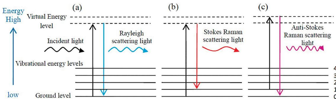
**Figure 4.** Diagram of the Rayleigh and Raman scattering processes:
