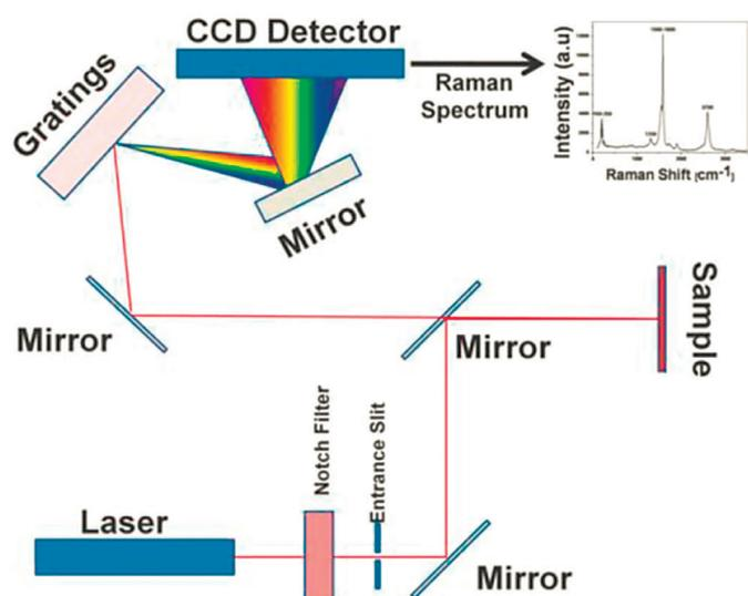
**Figure 5.** Principle scheme of the modern Raman spectrometer [36] spectroscopy, polarized Raman spectroscopy, stimulated Raman spectroscopy, transmission Raman spectroscopy, spatially offset Raman spectroscopy and hyper-Raman spectroscopy [30,36]. As a rule, the aim is an increase in sensitivity (for example, surface-enhanced Raman spectroscopy), improvement of spatial resolution (Raman microscopy) or acquisition of a very specific information (resonance Raman scattering).
